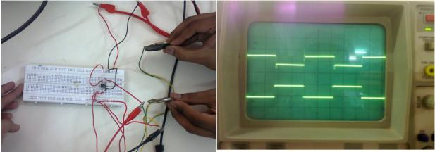
Fig. 4. Experimental setup of ANC using op-amp 741
