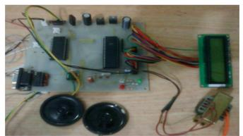
Fig. 6. ANC using microcontroller and ADC & DAC circuits
