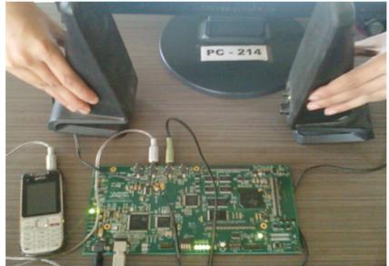
Fig. 7. ANC using DSP TMS320C6713
